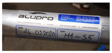
Separate all sections named M1 from these named M2, put them around their final installation places. There will be 5 sections called M1 and 5 sections M2. Letter "S" + number defines where given section goes in each mast.
