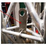
Run winch wire through upper pulley system. To do that unscrew upper C-channel as shown in photo, run the wire and put C-channel back on its place.
